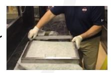
Place a new filter on top of the frame and then "snap" the cover in place by lining up the nipples and dimples on the sides of the filter.
